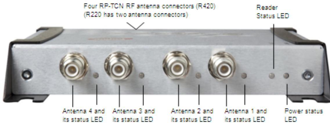
**Figure 5.2 Speedway R420 Antenna Ports and Status LEDs**
