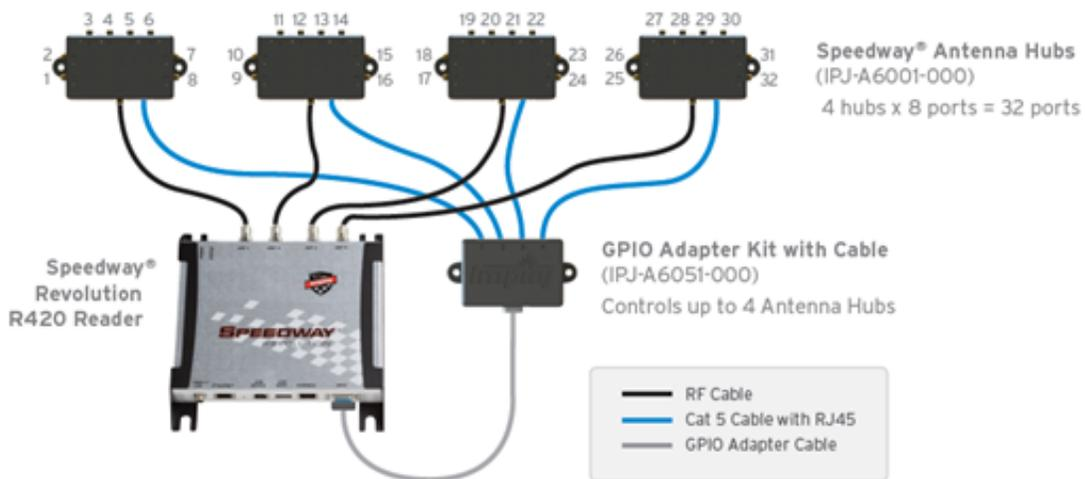
**Figure D.1** Speedway R420 Reader with four antenna hubs and GPIO adaptor for a total of 32 RF antenna ports.
