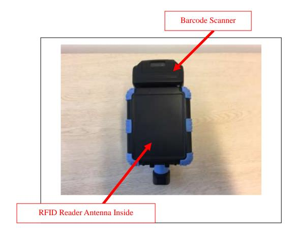
Figure 4-1 CS108-2 Reader Front View
